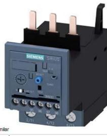
OVERLOAD RELAY 12.5...50 A FOR MOTOR PROTECTION SIZE S2, CLASS 10E FOR MOUNTING ONTO CONTACTORS MAIN CIRCUIT: SCREW TERMINAL AUX. CIRCUIT: SCREW TERMINAL MANUAL-AUTOMATIC-RESET
