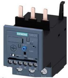
OVERLOAD RELAY 20...80 A FOR MOTOR PROTECTION SIZE S2, CLASS 10E FOR MOUNTING ONTO CONTACTORS MAIN CIRCUIT: SCREW TERMINAL AUX. CIRCUIT: SCREW TERMINAL MANUAL-AUTOMATIC-RESET
