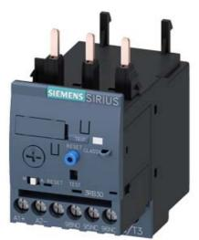
OVERLOAD RELAY 10...40 A FOR MOTOR PROTECTION SIZE S0, CLASS 10 CONTACTOR ASS. MAIN CIRCUIT: SCREW CONN. AUX.CIRCUIT: SCREW CONN. MANUAL-AUTOM.-RESET
