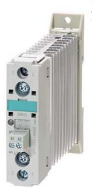
SEMI-COND. CONTACTOR 3RF2,1-PH. AC51 20 A 40 DEG. C 48-460 V / 4-30 V DC SCREW CONNECTION
