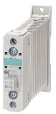
SEMI-COND. CONTACTOR 3RF2,1-PH. AC 51 20 A 40 DEGREES C 48-460 V / 24 V DC SHORT-CIRC. RESIST. WITH B-MCB
