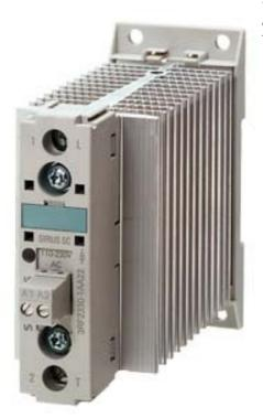
SEMI-COND. CONTACTOR 3RF2,1-PH. AC51 30 A / AC15 15A 40 DEG. C 48-460V / 4-30V DC SCREW TERMINAL INSTANTANEOUS SWITCHING
