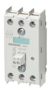
SOLID STATE RELAY 3-PHASE 3RF2 55 A 40 DEG. C 48-600 V / 4-30 V DC 2-PHASE CONTROLLED SCREW TERMINALS BLOCKING VOLTAGE 1200 V
