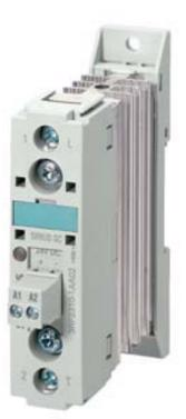
SEMI-COND. CONTACTOR,3RF2, 1-PH AC 51 10 A / AC15 6A 40 DEG. C 48-460 V / 24 V DC INSTANTANEOUS SWITCHING
