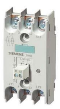
SOLID STATE RELAY 3-PHASE 3RF2 55 A 40 DEG. C 48-600 V / 4-30 V DC 3PH.-CONTROLLED RING TERMINAL LUG BLOCKING VOLTAGE 1200 V
