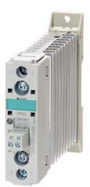
SEMI-COND. CONTACTOR 3RF2,1-PH. AC51 20A 40 DEGREE C 48-460 V / 4-30 V DC LOW NOISE
