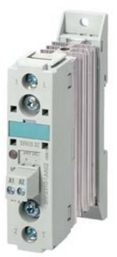
SEMI-COND. CONTACTOR 3RF2,1-PH. AC 51 10 A / AC15 6A 40 DEG. C 48-600 V / 24 V DC INSTANTANEOUS SWITCHING
