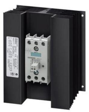
SEMI-CONDUCTOR CONTAC.3-PH.3RF2 AC51 50A 40 DEG. C 48-600V / 230V AC 3-PHASE CONTROLLED SCREW TERMINAL BLOCKING VOLTAGE 1200V
