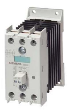
SEMI-CONDUCTOR CONTAC.3-PH.3RF2 AC51 10A 40 DEG. C 48-600V / 230V AC 3-PHASE CONTROLLED SCREW TERMINAL BLOCKING VOLTAGE 1200V
