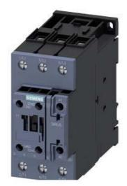
CONTACTOR,AC3:37KW/400V, 1NO+1NC, 20-33V AC/DC, WITH VARISTOR, 3-POLE, SIZE S2, SCREW TERMINAL
