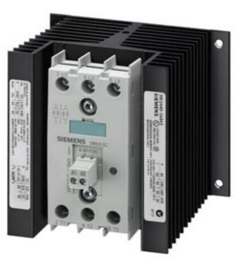
SOLID-STATE CONTACT.3PHASE 3RF2 AC51 40A 40 DEG. C 48-600V / 110V AC 2-PHASE CONTROLLED SCREW TERMINAL BLOCKING VOLTAGE 1200V
