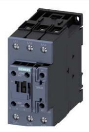
CONTACTOR,AC3:18.5KW/400V, 1NO+1NC, 20-33V AC/DC, WITH VARISTOR, 3-POLE, SIZE S2, SCREW TERMINAL
