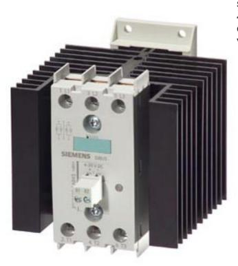
SOLID-STATE CONTACT.3PHASE 3RF2 AC51 20A 40 DEG. C 48-600V / 110V AC 3-PHASE CONTROLLED SCREW TERMINAL BLOCKING VOLTAGE 1200V
