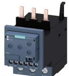
MONITORING RELAY ATTACHABLE TO CONTACTOR 3RT2. SIZE S00 BASIC, ANALOG ADJUSTMENT APPARENT CURRENT MONITORING 8 - 80 A, 50-60 HZ, 2-PHASE SUPPLY 24-240 V AC/DC 1 CO CONTACT MONITORING FOR CURRENT OVERSHOOT/UNDERSHOOT PHASE FAILURE, WIRE BREAK WITH OR W/O ERROR LOG ON-DELAY 0-60 S SPURIOUS PEAK SUPPR.0-30 S SWITCHING HYSTERESIS 6% SCREW TERMINAL
