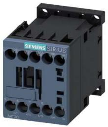
CONTACTOR, AC-3, 7.5KW/400V, 1NC, AC 230V, 50/60 HZ, 3-POLE, SZ S00 SCREW TERMINAL
