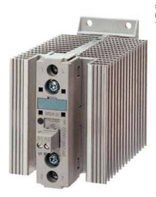
SEMI-COND. CONTACTOR 3RF2,1-PH. AC51 50A 40 DEGREES C 48-460V / 24V AC/DC SCREW TERMINAL
