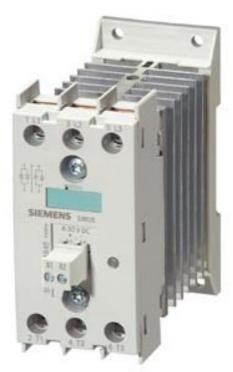
SOLID STATE CONTACTOR 3-P. 3RF2 AC51 10 A 40 DEG. C 48-600 V / 4-30 V DC 2PH.-CONTROLLED SCREW TERMINAL BLOCKING VOLTAGE 1200V
