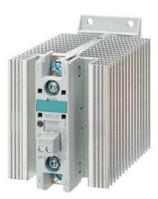
SEMICONDUCTOR RELAY 3RF2, 1-PH. AC51 50A 40 DEGREES C 48-460V/4-30V DC RING TERMINAL
