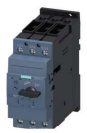
CIRCUIT BREAKER, SIZE S2, FOR MOTOR PROTECTION, CLASS 10, A-RELEASE 28...36A, N-RELEASE 520A, SCREW TERMINAL, STANDARD BREAKING CAPACITY
