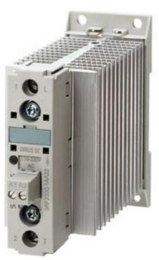
SEMI-COND. CONTACTOR 3RF2,1-PH. AC 51 30A / AC15 15A 40 DEG. C 48-600 V / 24 V DC INSTANTANEOUS SWITCHING
