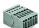
Item no.: 769-610/001-000 1-conductor male connector; Snap-in mounting feet; 4 mm 2 ; Pin spacing 5 mm; 10-pole
