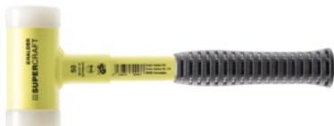
The head of the SUPERCRAFT mallet is filled with steel shot. This means that when the workpiece is impacted, the energy of the shot is transferred with a slight delay. The reduced rebound allows the impact energy to be absorbed, resulting in extremely powerful impact without vibration which is much easier on your joints. Additionally, an advantage over steel mallets is the reduced noise level.
